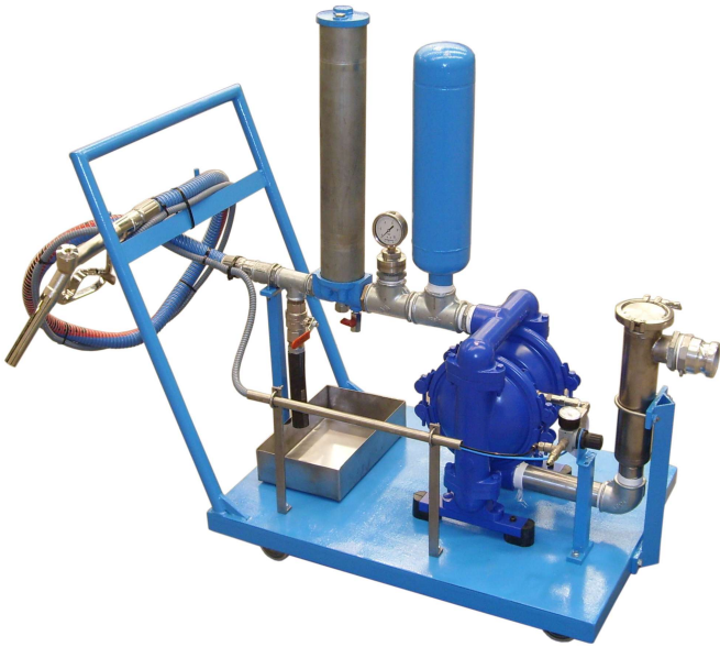
Circulation equipment with membrane pump, vibration absorber pre-filter, 20" cuno filter, 1 1/2" pre-filter and dispenser gun
