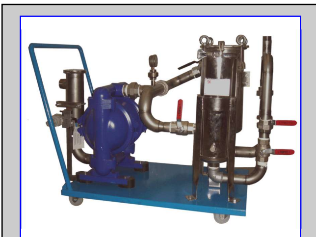
Circulation equipment with membrane pump which drives fluids to bag filter or stainless steel case with three 10" cuno filter
