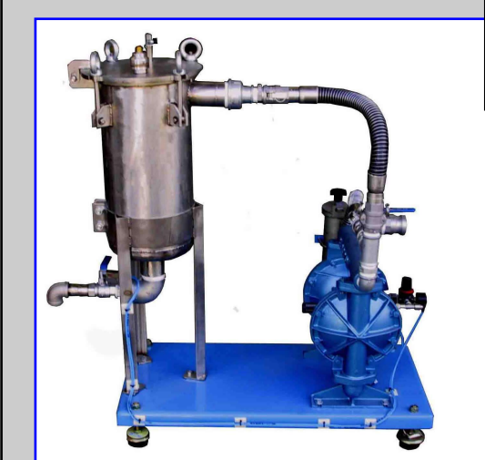
Circulation equipment with membrane pump and bag filter
