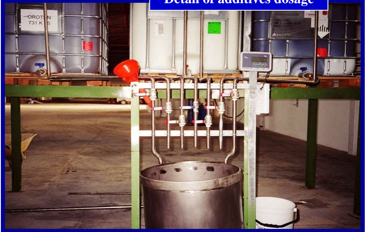
Detail of additives dosage
